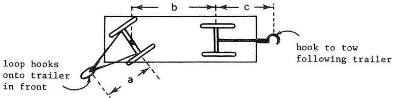
Problem: how should the dimensions a, b and c be proportioned so as to make the train follow as nearly as possible the path taken by the tractor?
